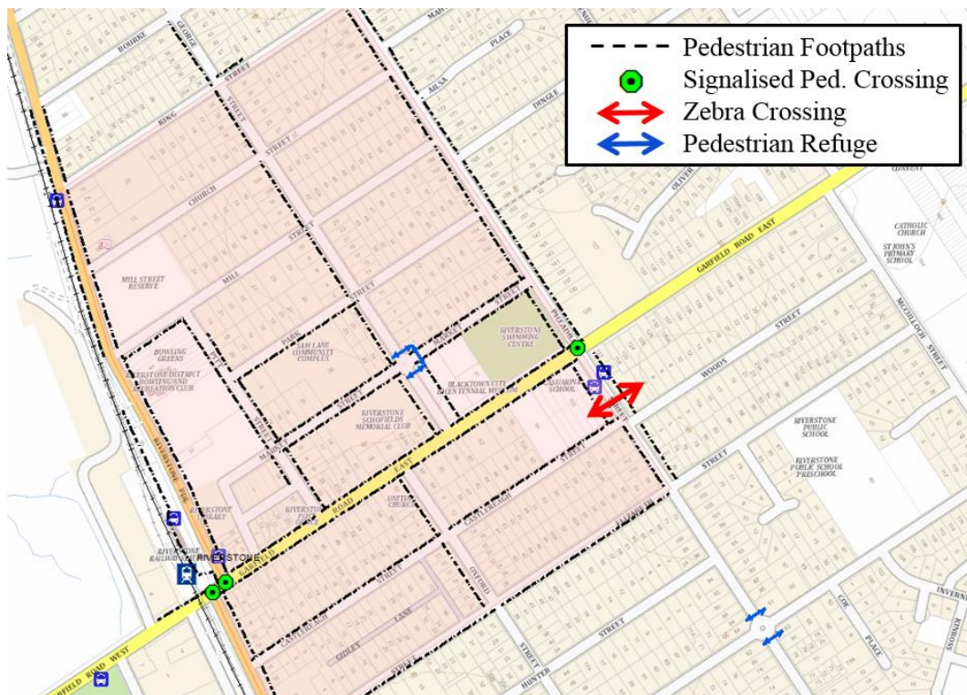
Figure 16 Existing pedestrian facilities
